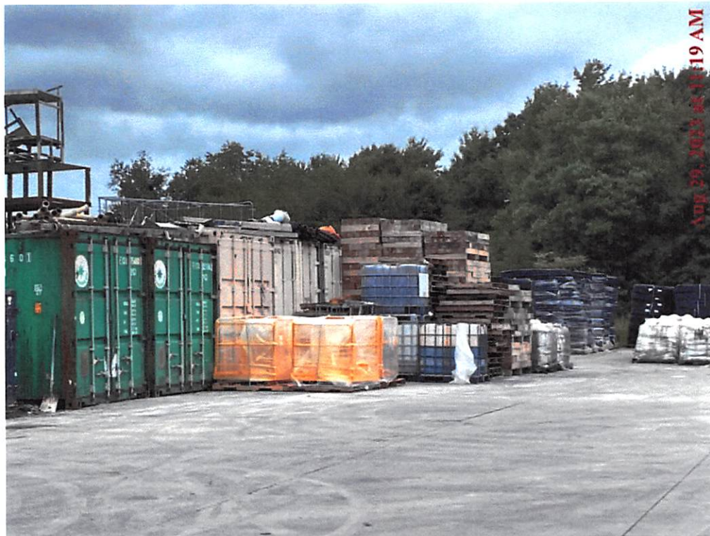
08/29/23 Totes with product and without secondary containment.
