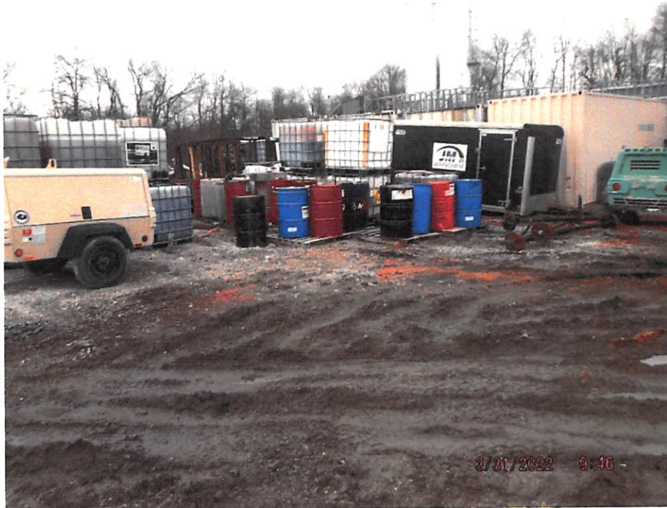
03/31/22 Spills on the ground and unlabeled totes and drums without secondary containment.
