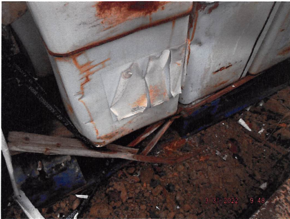
03/31/22 Damaged containers leaking onto ground.
