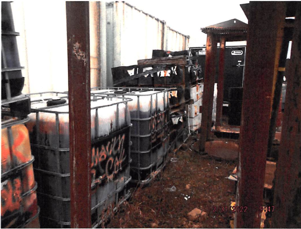
03/31/22 Old drums and deteriorating containers without secondary containment.
