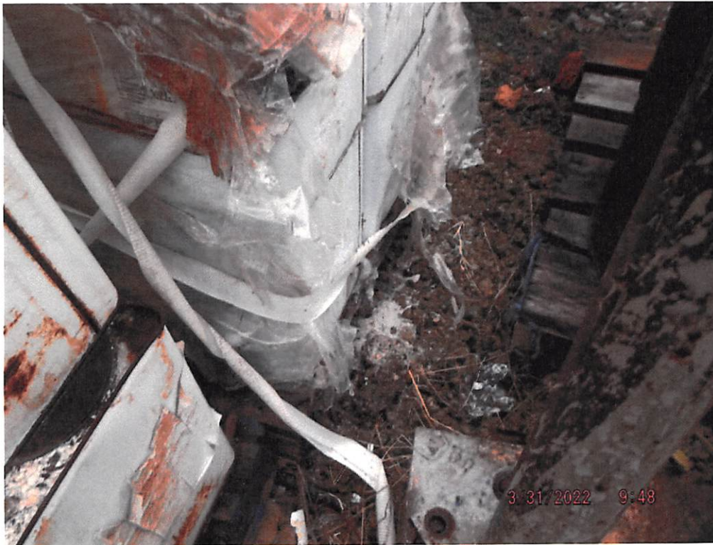
03/31/22 Damaged plastic containers leaking solids onto ground.
