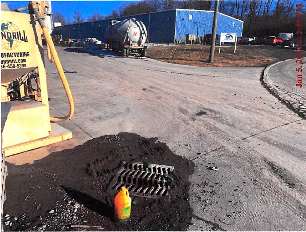
01/05/24 Green dye was put in the storm drain.
