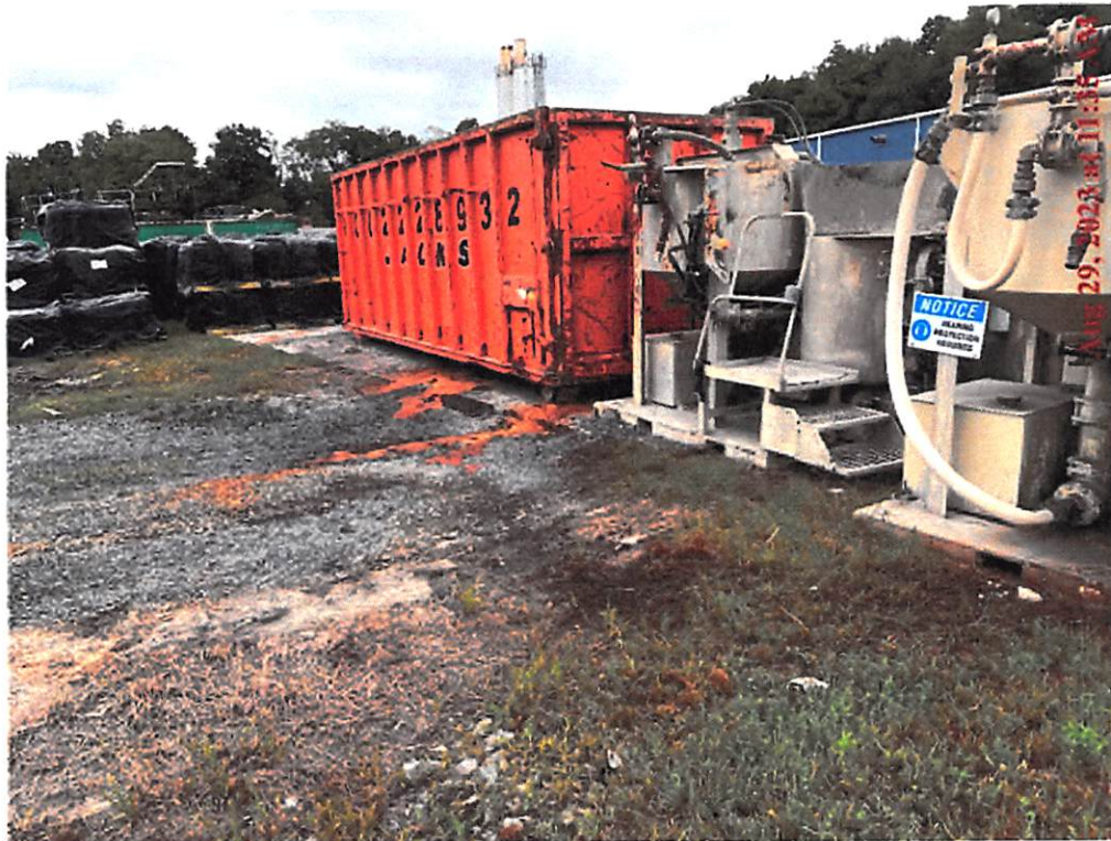
08/29/23 Unknown liquid leaking from dumpster and petroleum staining.
