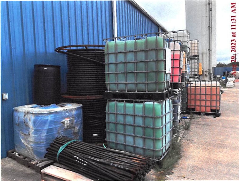
08/29/23 Drums and totes with product and without secondary containment.
