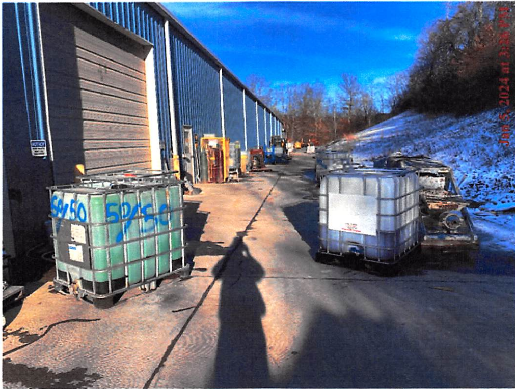
01/05/24 Containers with product were without secondary containment.
