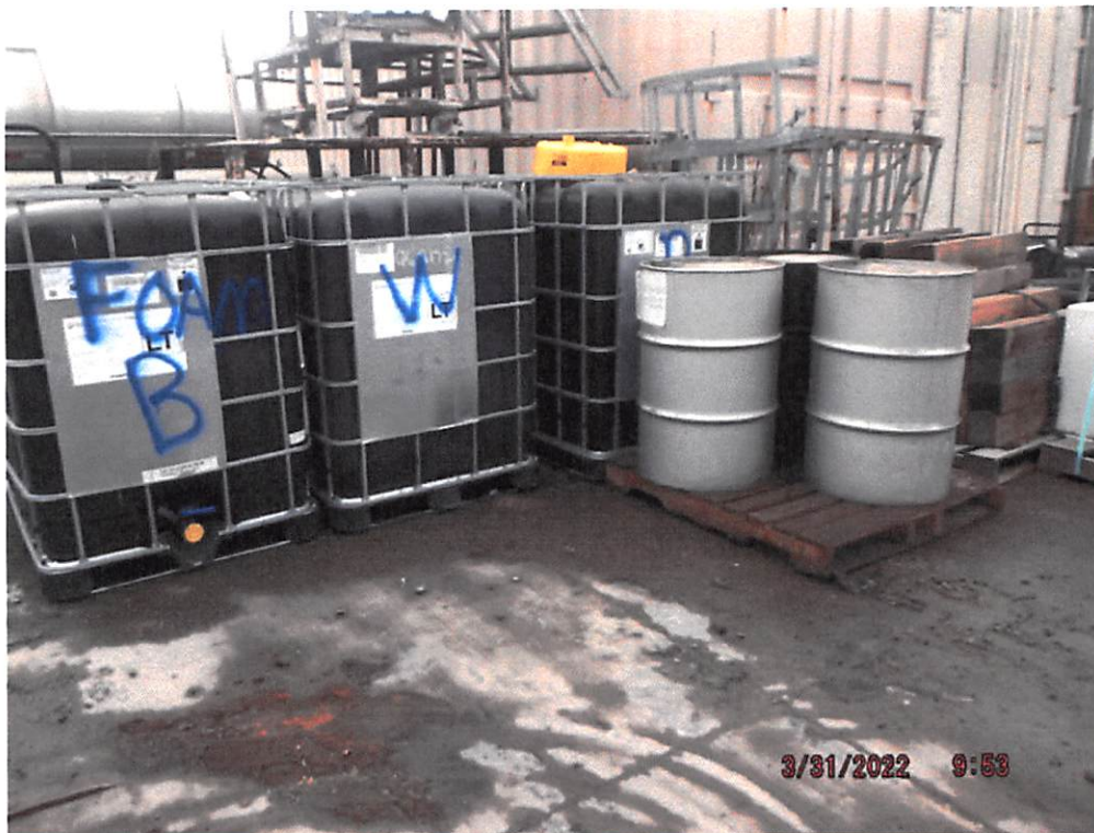
03/31/22 Totes and drums without secondary containment.
