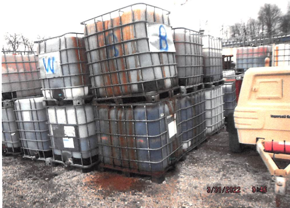
03/31/22 Unlabeled totes without secondary containment and spills on the ground.
