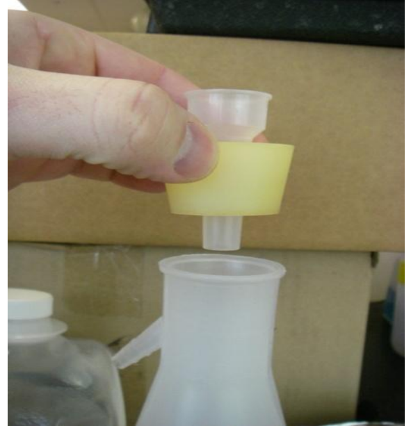
Figure 66. Photo of the insertion of rubber stopper into flask with plastic funnel already inserted through rubber stopper.
