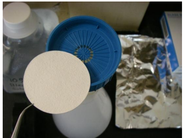
Figure 68. Photo of the GF/F filter being placed on top of support screen with forceps.
