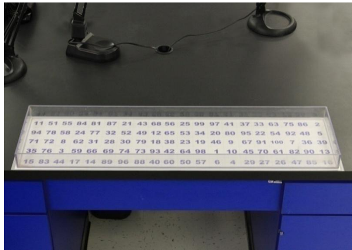
Figure 53. Photograph of a Home-Made Gridded Sorting Tray featuring a random number matrix on the bottom.
