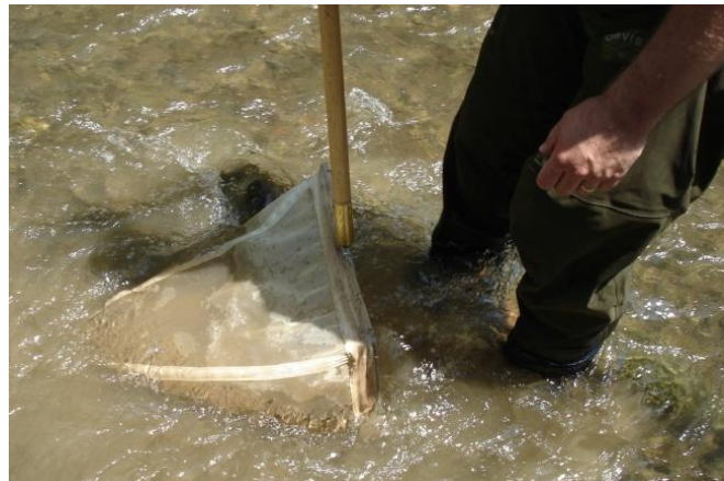
Figure 46. Photograph of the Kicking process in front of the net.
