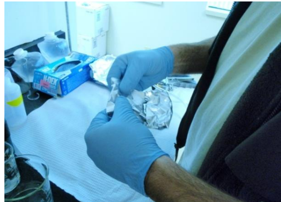
Figure 72. Photo of the filter disk being wrapped loosely in one 4"X4" aluminum foil square to prevent loss of algal cells via compression and smearing
