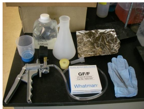
Figure 64. Photo of the materials used to filter a Golden Algae sample.
