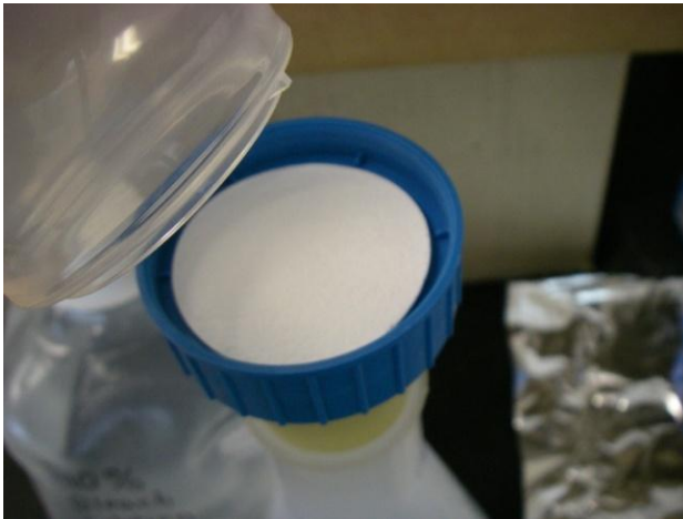
Figure 67. Photo of cup being removed to access the prepackaged filter for removal.
