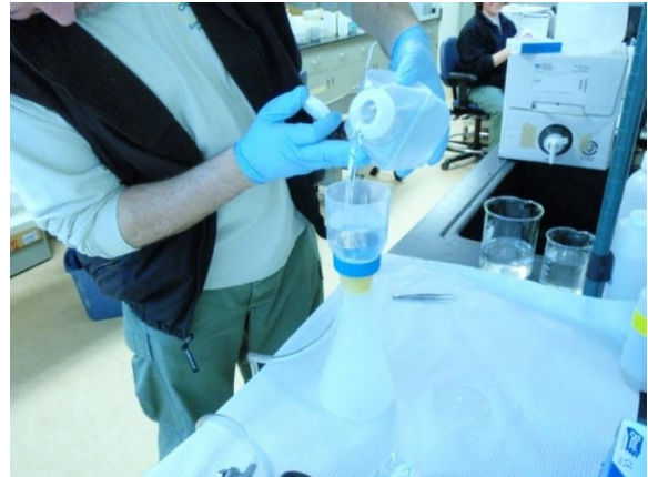
Figure 70. Photo of the pouring of a 250 mL sample into filter cup.
