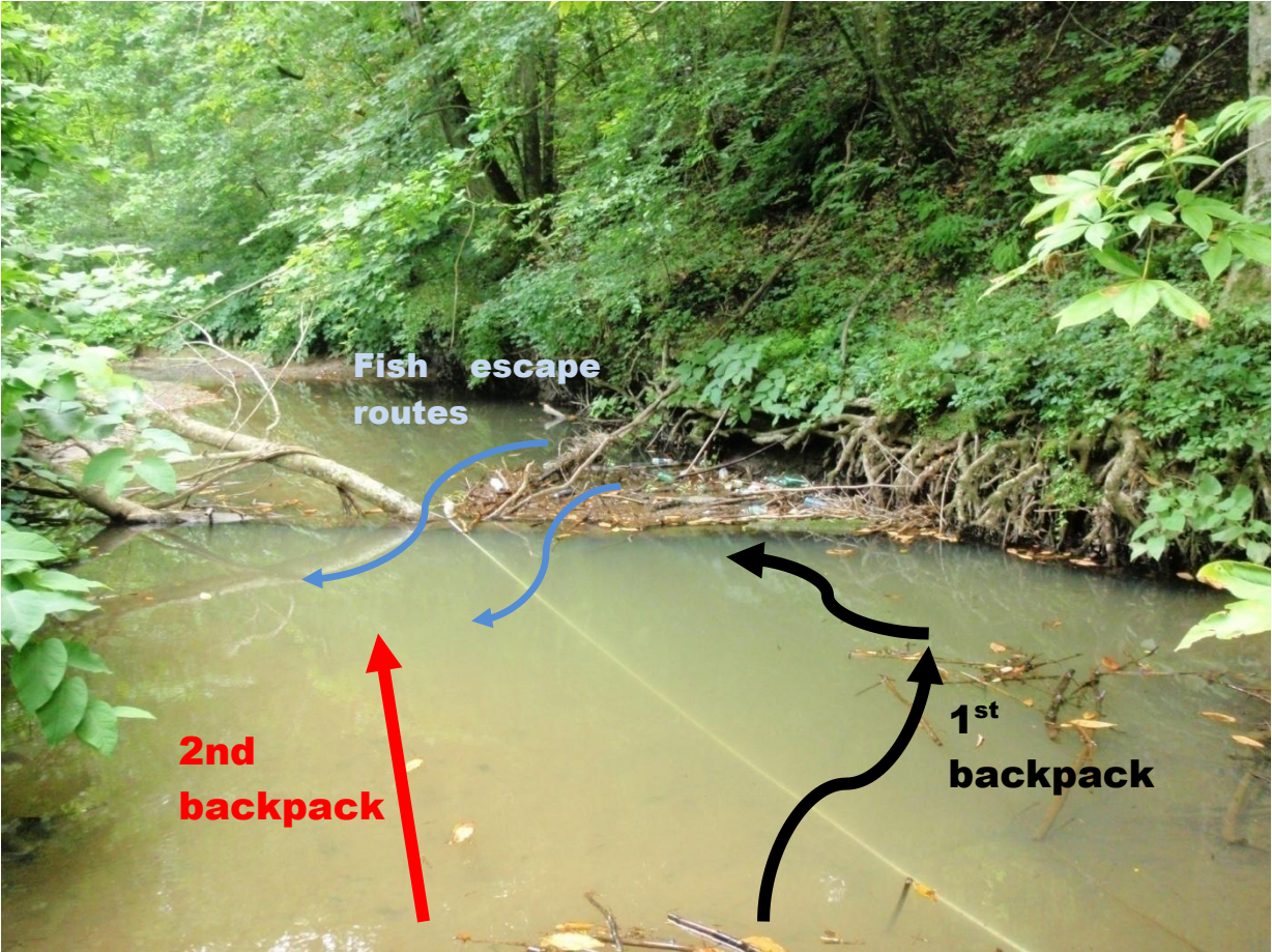
Figure 60. Technique for sampling a deep, narrow stream with two backpacks, looking upstream.
