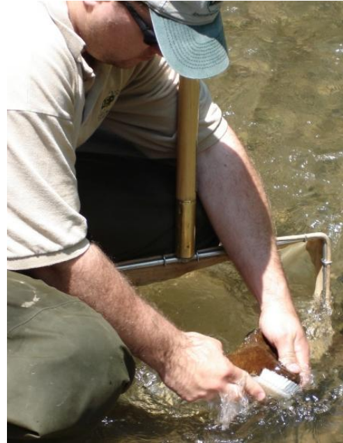
Figure 45. Photograph of the Brushing process in front of the net.
