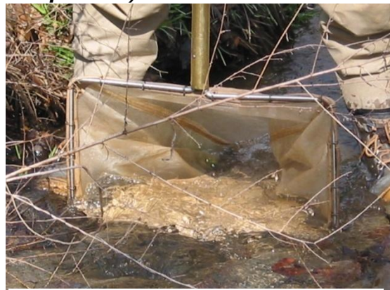
Figure 44. Photo of Rectangular Frame Dip Net being placed on stream bottom
