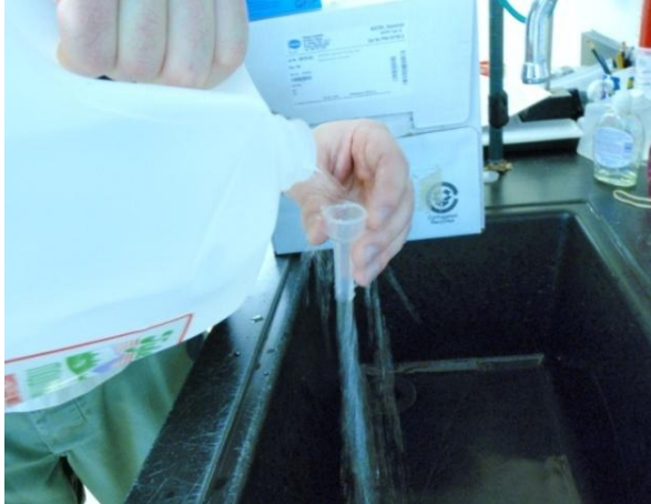
Figure 75. Photo of forceps being rinsed with deionized (DI) water.
