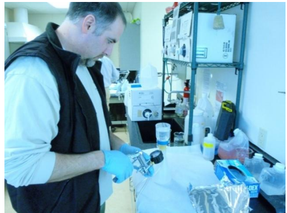
Figure 71. Photo of monitoring the pump pressure while filtering sample – keep pressure under 5 psi.
