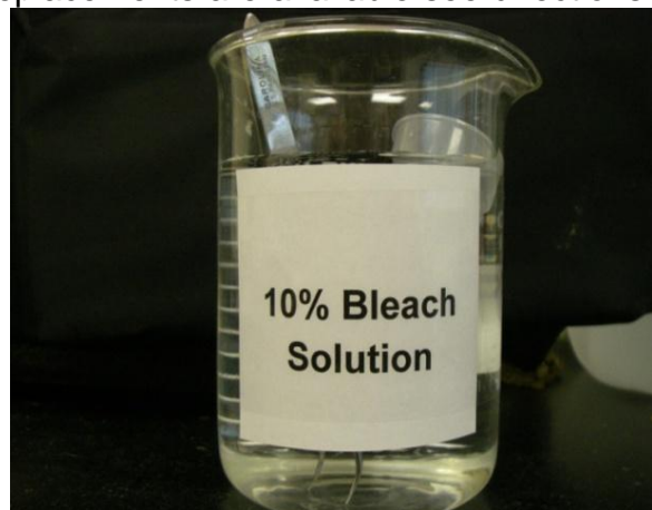
Figure 73. Photo of Forceps and small plastic funnel soaking in 10% bleach solution for 1 minute.
