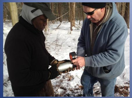
Soil sampling along TGP 300 Line commissioned by DRN indicates soils in TWS more compacted than specs. for an earthen dam. (Meliora Tech Memo, 2/2013)
