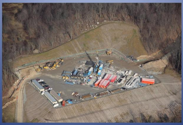
Well pad located in Hop Bottom, Pennsylvania. The pipe for the gathering line can be seen being laid off to the right of the pad. At this location there are 3 pads located within a mile and a half of each other, all to be connected together with gathering lines.
